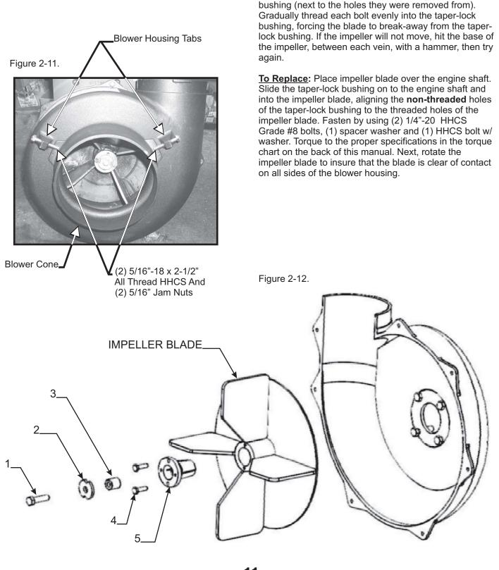
2-12 Impeller Blade Removal/Replacement
